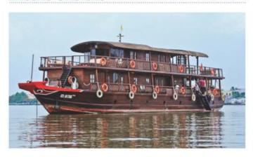
All three Bassac are built of wood according to the tradition of the rice barges of the Mekong delta, with amendments where safety standards require. Bassac I actually once was a rice barge, which we bought and overhauled into the cozy cabin cruiser it is today, and although Bassac II and III are entirely new hull designs, more adapted to their present purpose, they were built with the same craftsmanship and according to the same tradition.
